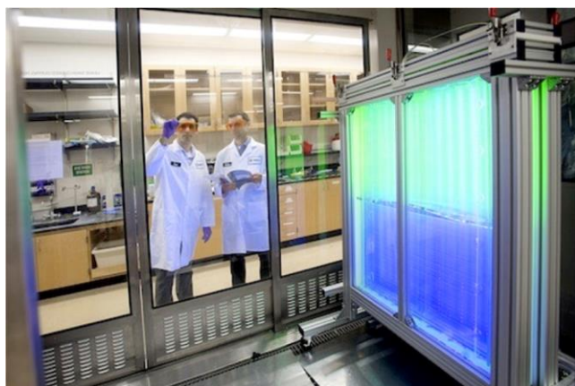
Figure 3. Process-scale photoredox flow reactor at Merck. Photo courtesy of Merck and Co. Inc. Copyright 2016 American Chemical Society. 27,49
