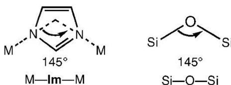
Figure 5. Zeolite-type Tetrahedral Topology Resulted from 145° between metals in ZIF (Left) or the Si in zeolites (Right). (Figure adapted with permission from Ref. 15. Copyright (2010) American Chemical Society.)
