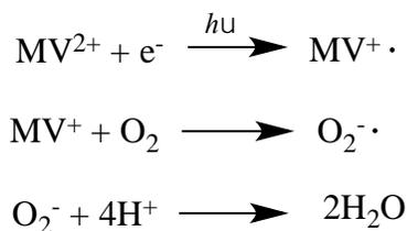
Scheme 3 – the half-reaction occurring at the photoanode of the biovoltaic cell developed by Kothe et al.<sup>35</sup>
