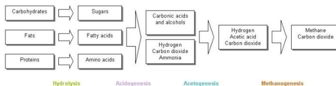
**Figure 2: Stages of Anaerobic Digestion<sup>15</sup>**
