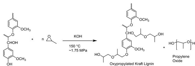
Scheme 3. Kraft lignin oxypropylation reaction
