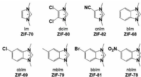
Figure 4. Substituents on the Imidazolate Organic Linker for Selective Absorption of CO<sub>2</sub> (Figure adapted with permission from Ref. 11. Copyright (2009) American Chemical Society.)
