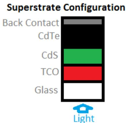
Figure 2: Basic schematic of CdTe Thin Film photovoltaic cell. Design interpreted from Romeo et al. (2004)<sup>3</sup>. (TCO=Transparent Conducting Oxide)
