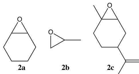
Figure 2. Comparison of epoxides used, (2a) Cyclohexene Oxide. (2b) Propylene Oxide. (2c) Limonene Oxide.
