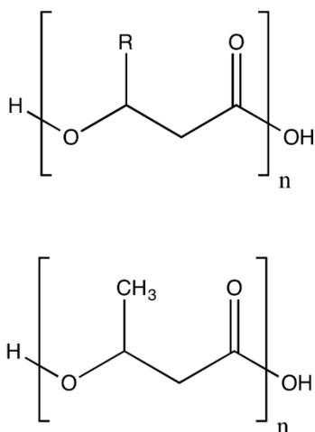
Figure 1. Chemical structure of polyhydroxyalkanoates. Top: General structure of PHAs. Bottom: Structure of PHB
