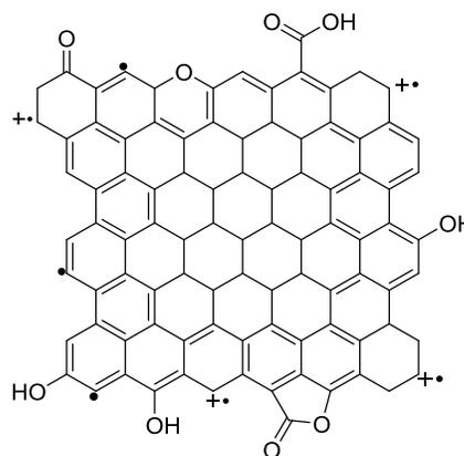
**Figure 1. AC chemical structure responsible for its hydrophobicity (based on structure as proposed by Mochida)<sup>19</sup>**
