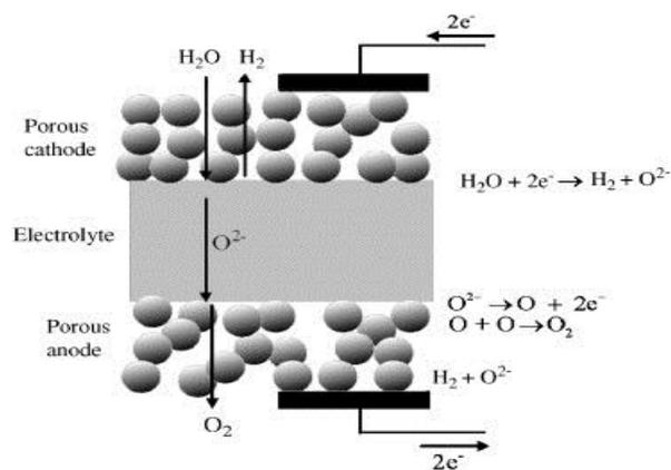
Figure 3. Schematics of SOEC hydrogen production [24]
