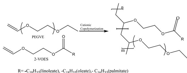
Scheme 3. Synthesis of the SBPS copolymer, where R is soybean fatty acid component. Adapted from Popadyuk *et al*<sup>15</sup>
