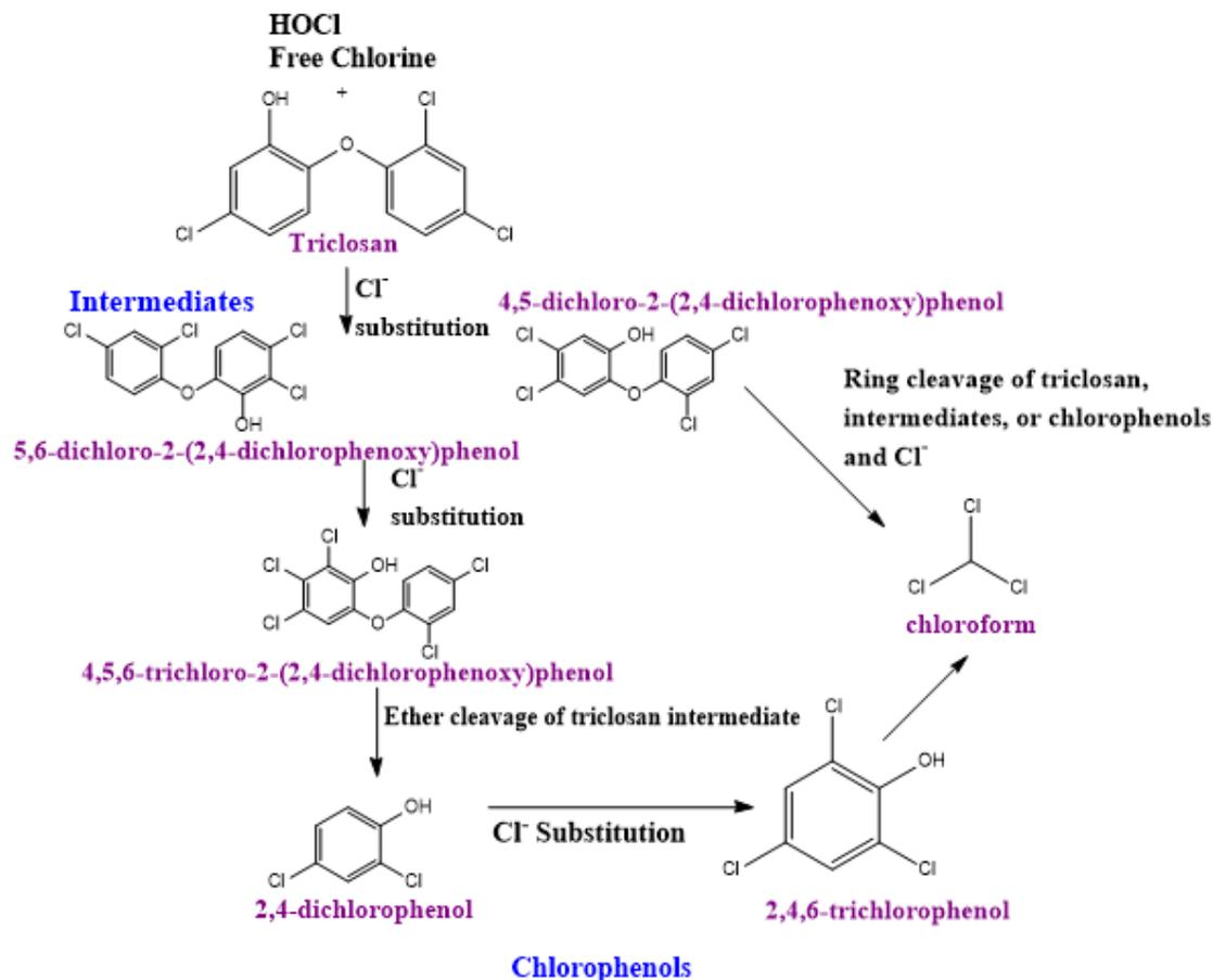
**Scheme 1.** Reaction scheme showing reaction mechanisms and chemical structures for triclosan and its decay products
