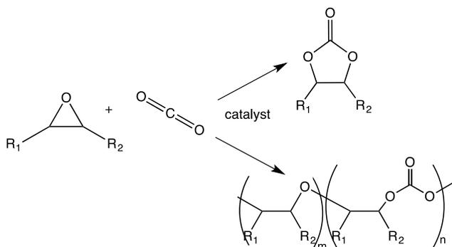
Scheme 1. General Copolymerization Reaction<sup>4</sup> to yield either a cyclic carbonate (top product) or a polycarbonate with possible ether linkages.
