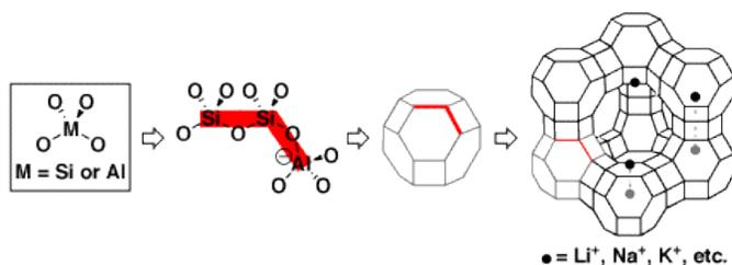
Figure 1. From Silica and Aluminum to the Zeolite Framework. (Figure from Professor T. Poon's research website<sup>8</sup>.)
