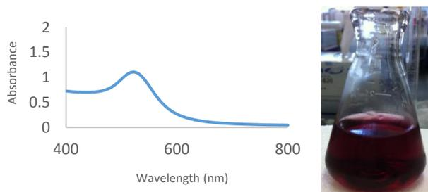
Figure 1. UV/vis of 10 nm glucose reduced AuNPs, demonstrating the surface plasmon resonance band
