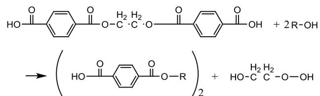
Methanolysis is performed in excess methanol at high pressure and temperature (2-4MPa and 453K-553K) along with a transesterification catalyst, which is usually zinc
