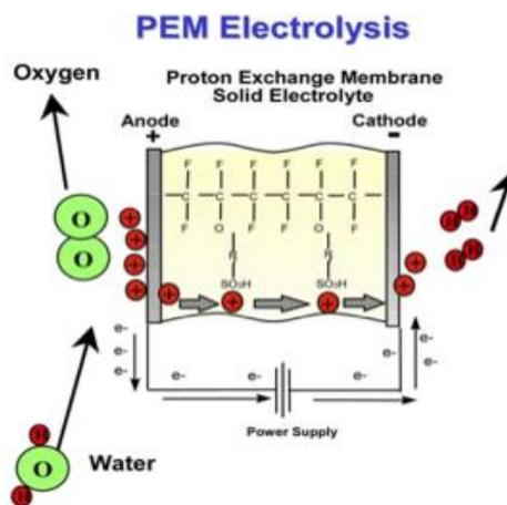
Figure 2. Schematic representation of PEM electrolysis [22]
