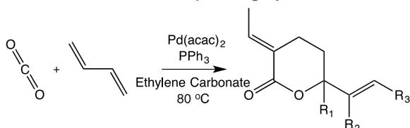
Scheme 2. First reaction in the process to obtain the lactone intermediate before subsequent copolymerization.<sup>1</sup>
