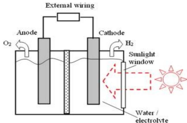
Figure 4: Components of a photoelectrolysis or photochemical unit [35]
