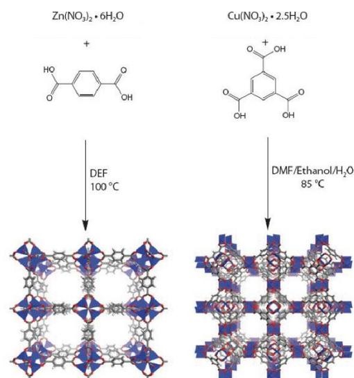
Figure 2. From Hydrated Metal Salts and Organic Linkers to Metal Organic Framework (Figure adapted from Sigma Aldrich<sup>9</sup>)
