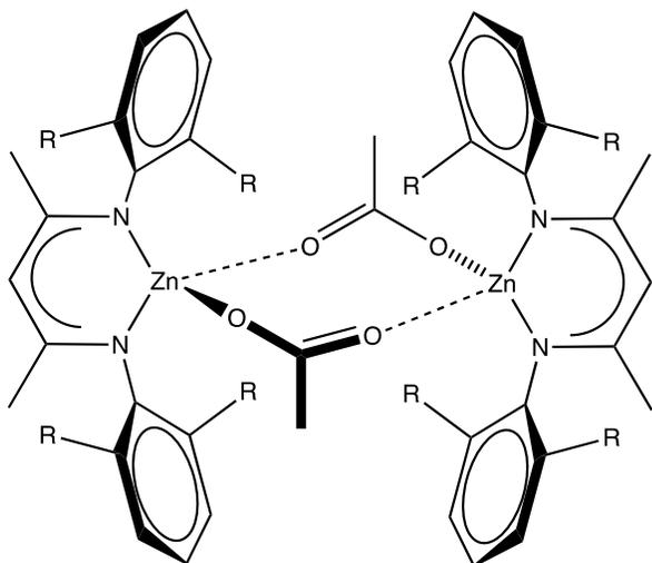
Figure 1. Loosely associated dimer of the  $\beta$ -diimine zinc catalyst.<sup>15</sup> This is the most active form of the catalyst.
