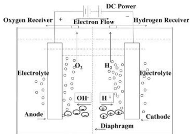
Figure 1. A schematic illustration of a basic water electrolysis system [15]
