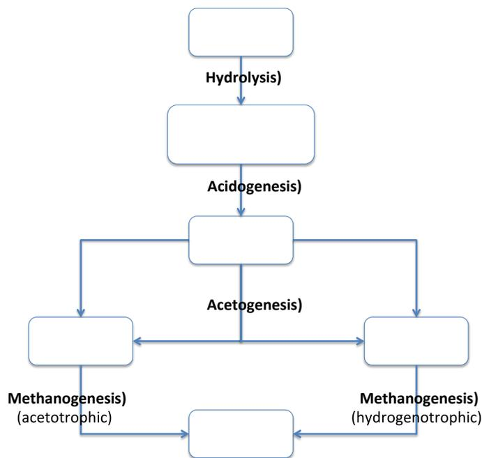
Figure 2: Schematic diagram of anaerobic digestion processes.
