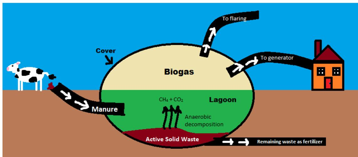
**Figure 1.** The anaerobic decomposition of manure in a lagoon forming methane biogas, to be used as an alternative energy source or flared to the environment. Remaining manure can be used as fertilizer.
