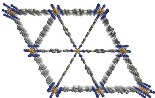
Figure 3. The Sharply Angled and Flat Pore Walls of Fe<sub>2</sub>(BDP)<sub>3</sub> Framework (Figure adapted with permission from AAAS<sup>12</sup>).
